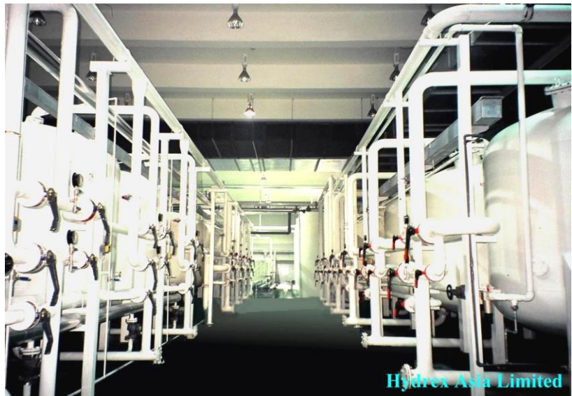
Filter arrays for one of the largest soft drink bottling plants in the world.
